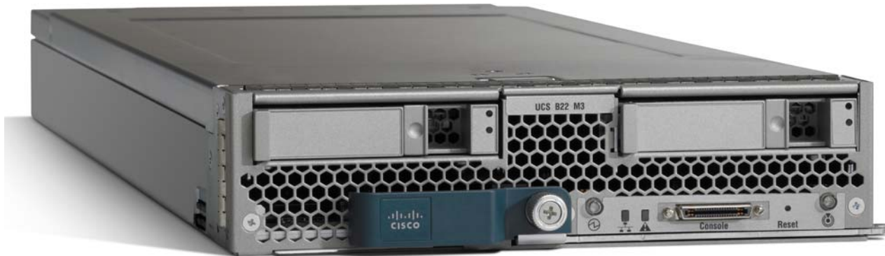
Figure 1 Cisco UCS B22 M3 Blade Server
